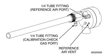
Figure 2-11. Oxygen Probe Gas Connections
